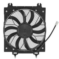
To prevent damage if a cooling fan gets blocked, the circuit powering the fan needs a time-delay type fuse with the correct amperage rating. This installation uses 1x suction fan - part number FAN0606 (F27P-12E8004-41S). The nominal running current is 7 amps.
